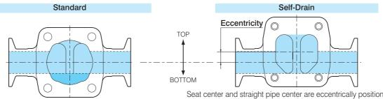
The valve seat is on the same centerline with straight pipe.
