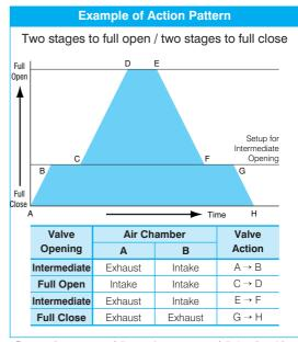
Patterns "one stage to full open / two stages to full close" and "two stages to full open / one stage to full close" are available as well.
