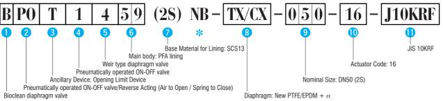
Above is the coding system for our products. An additional code may be added in accordance with the combination of parts, option, special specifications, etc. Please contact us for any questions regarding the details of product coding.
